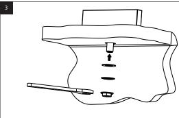
Tighten Mounting Pin with Locknut and washers
