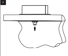
Connecting Underside of Mounting Pin to water supply line
